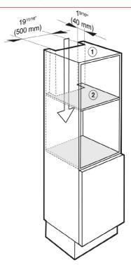
To ensure that the Combi Steam Oven has adequate ventilation, the following cut-outs measuring 19 11/16" x 1 9/16" (500 x 40 mm) must be made:
