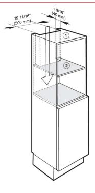
To ensure that the Combi Steam Oven has adequate ventilation, the following cut-outs measuring 19 11/16" x 1 9/16" (500 x 40 mm) must be made:
